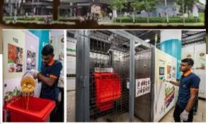
The food waste composting process is fully automatic. The waste just needs to be loaded onto the Eco Digester's conveyor lift and it will be processed within 24 hours.
